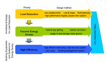
Figure 5 Schematic design flow of low carbon building
